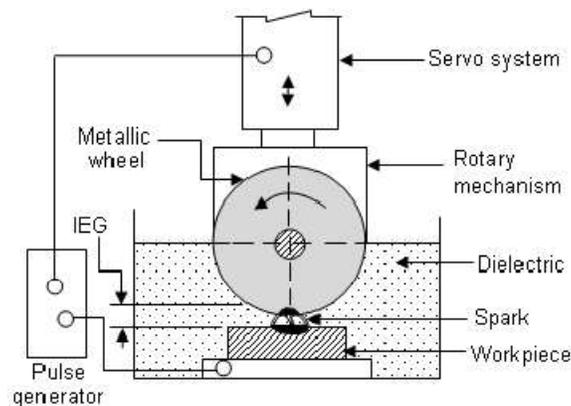
**Figure 1:** Schematic view of EDG
