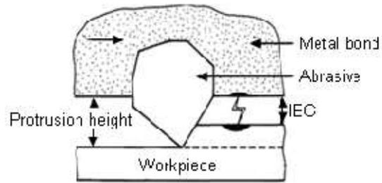
**Figure 2:** *Spark-erosion and abrasive abrasion in SAAG [15]*
