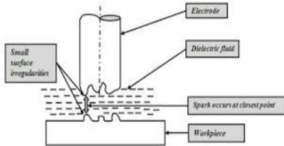
**Figure 1:** Material removal mechanism of electric discharge machining. [4]
