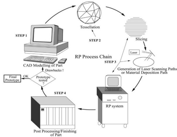
**Figure 4:** Process chain involved in AM Processes [19].
