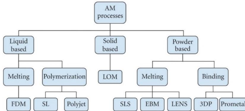
**Figure 2:** Three-dimensional printing processes. [9].
