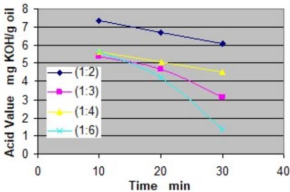
*Figure 2 Effect of molar ratio on esterification for temperature 40°C, 1% weight of catalyst concentrations using sonochemical method*
