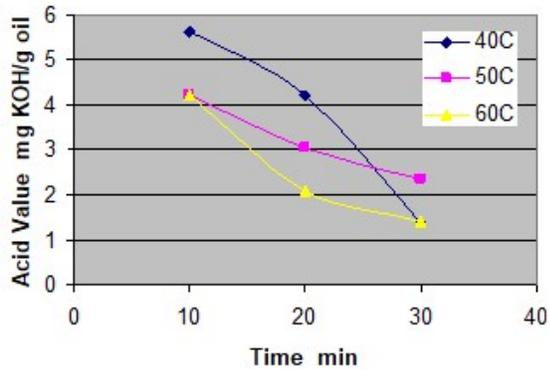
*Figure 1: Effect of temperature on esterification for 1:6 molar ratio, 1% weight of catalyst concentrations using sonochemical method*
