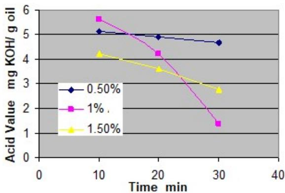
**Figure 3 Effect of catalyst concentration on esterification for 1:6 molar ratio, temperature 40<sup>0</sup>C using sonochemical method**
