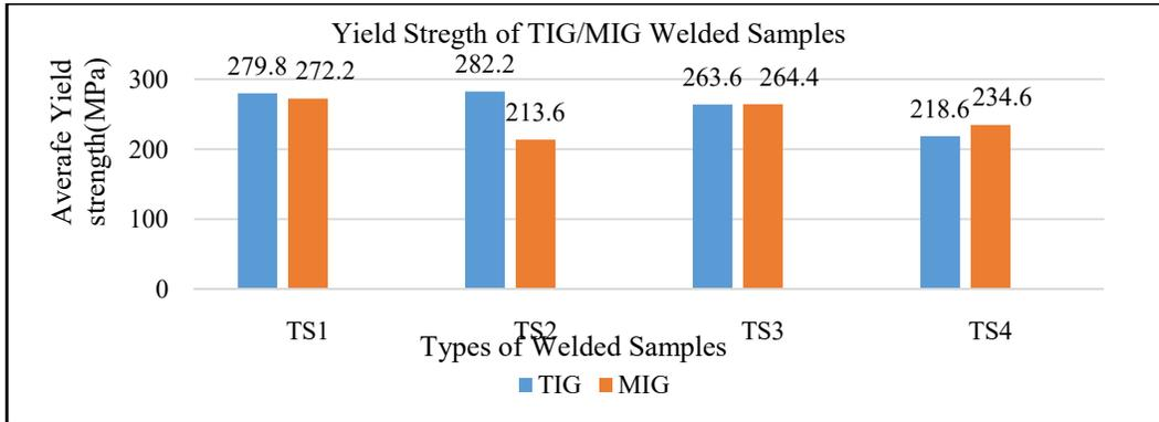
Figure 9: Comparative study of TIG and MIG welded joint for Yield Strength [5]
