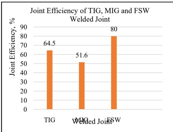
**Figure 5:** Tensile Properties of BM and Different Welded Joints [1]
