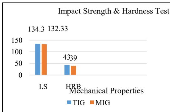
**Figure 3:** Comparison of hardness and impact strength of TIG & MIG welded Aluminum alloy [3]
