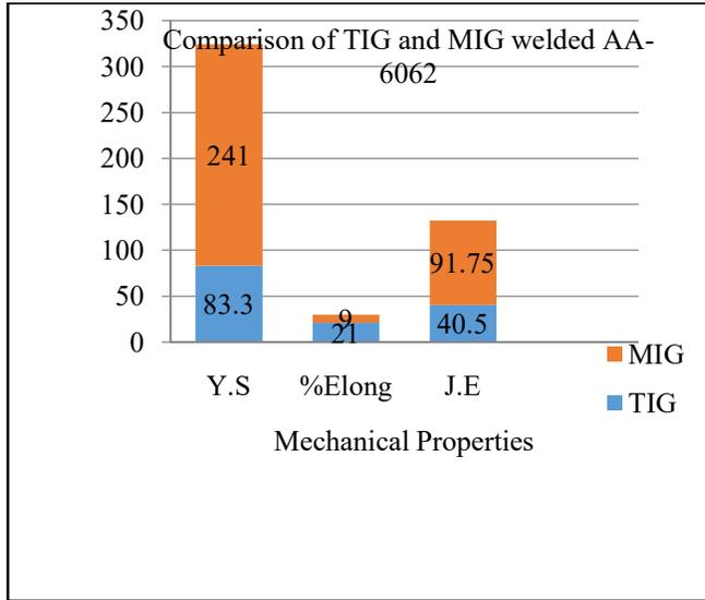
Figure 6: Comparison of mechanical properties of TIG & MIG welded AA-6062[4]
