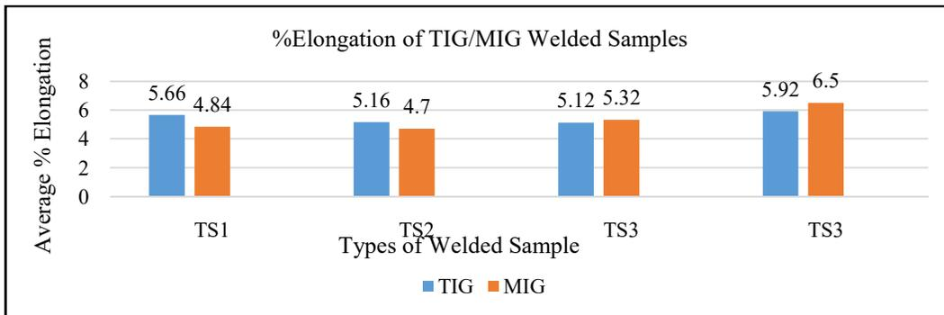
Figure 10: Comparative study of TIG and MIG welded joint for Average % Elongation [5]
