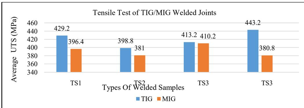
Figure 8: Comparative study of TIG and MIG welded joint for Tensile Test [5]
