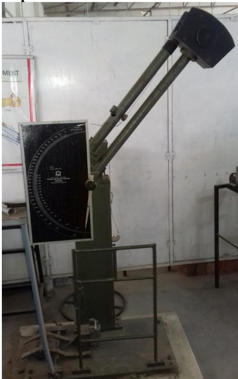
**Fig-Impact testing machine**
