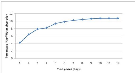
**Figure4:** Percentage of water absorption behaviors of betel nut powder/epoxy composites
