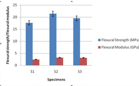
**Figure 2:** Flexural strength and flexural modulus of betel nut powder/epoxy composites
