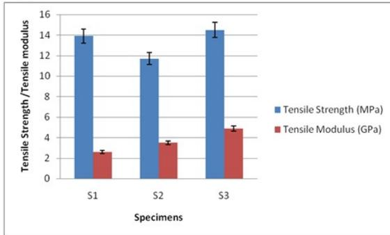
**Figure 1:** Tensile strength and tensile modulus of betel nut powder/epoxy composites
