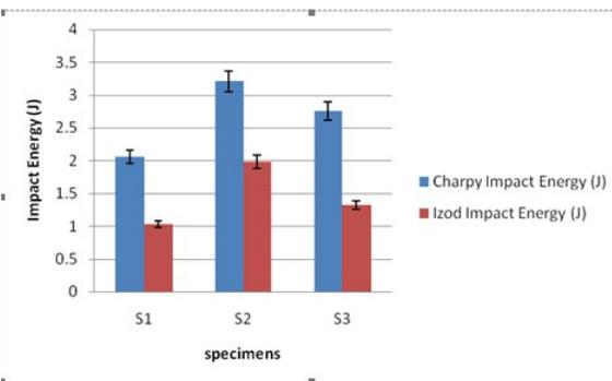
**Figure 3:** Charpy and Izod impact energy of betel nut powder/epoxy composites
