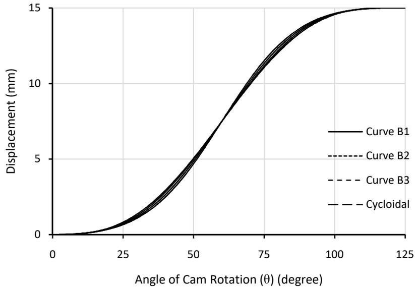
**Figure 1:** Simulated Follower Displacement of Cam Profileusing Six-Points Bézier curves
