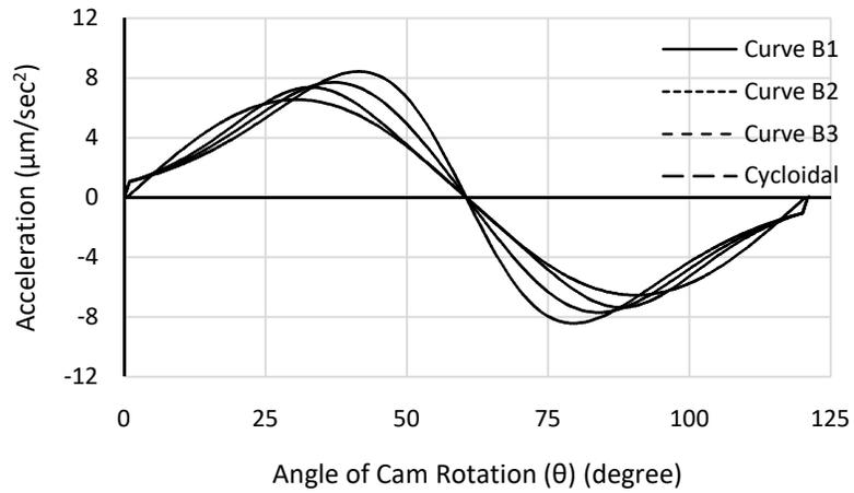
**Figure 3:** Acceleration Profiles of Roller Follower for Six-Points Bézier Curves
