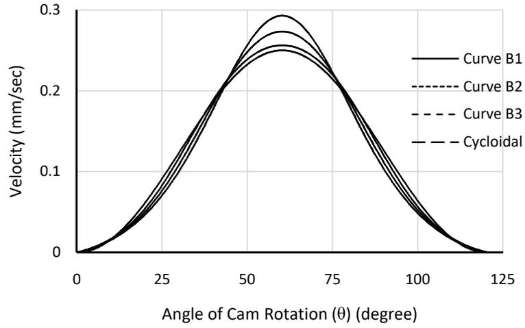
**Figure 2:** Velocity Profiles of Roller Follower for Six-Points Bézier Curves
