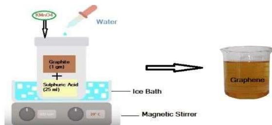
**Figure3:** Hummers methods of graphene
