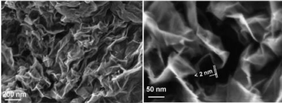
**Figure 4:** A SEM image aggregate reduced GO sheet[23]
