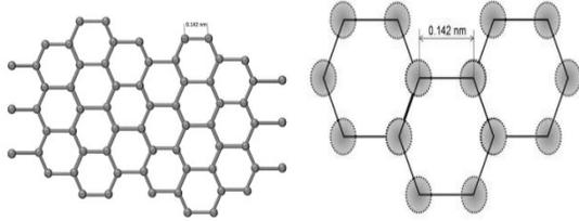
**Figure 1:** Graphene lattice structure of a honeycomb carbon atom in 0.142 nm length [4]
