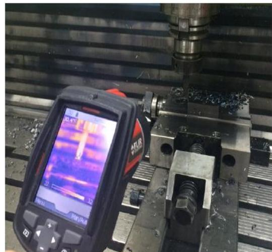
Fig. 1. Monitoring the temperature using infrared camera
