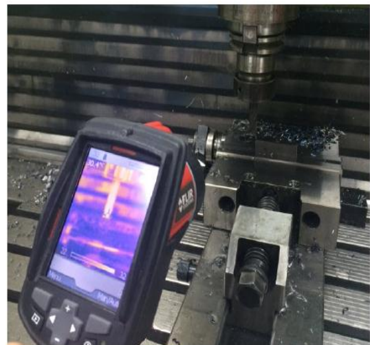
Fig. 1. Monitoring the temperature using infrared camera
