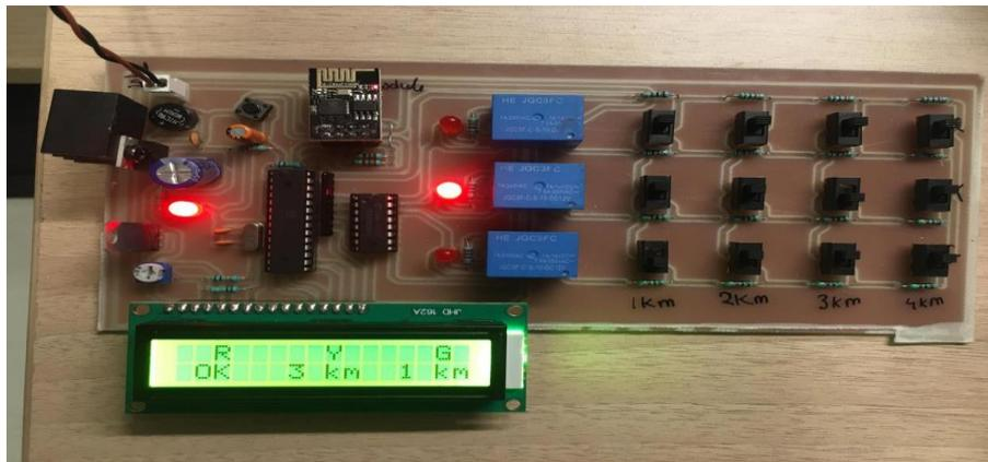
**Figure 12** Hardware on simulation of no fault in the cable
