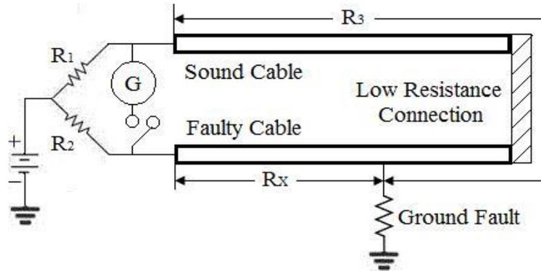
**Figure 4** Murray loop test circuit for short circuit fault
