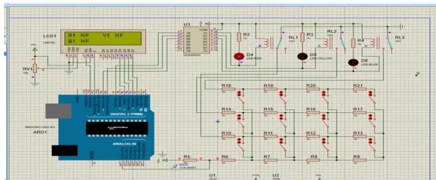
**Figure 8** Simulation of fault at 2 km of Y cable
