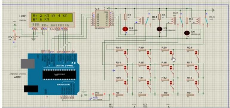
**Figure 11** Hardware showing simulation of fault at 3 km of Y and 1 km of G cable
