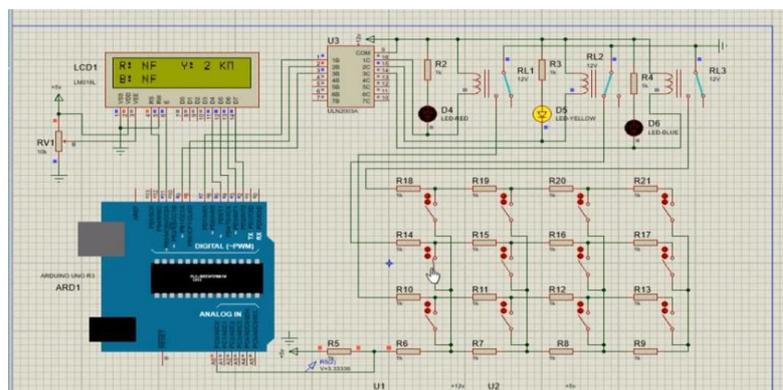
**Figure 10** Simulation of fault at 2 km of R, 4 km of Y and 6 km of G cable
