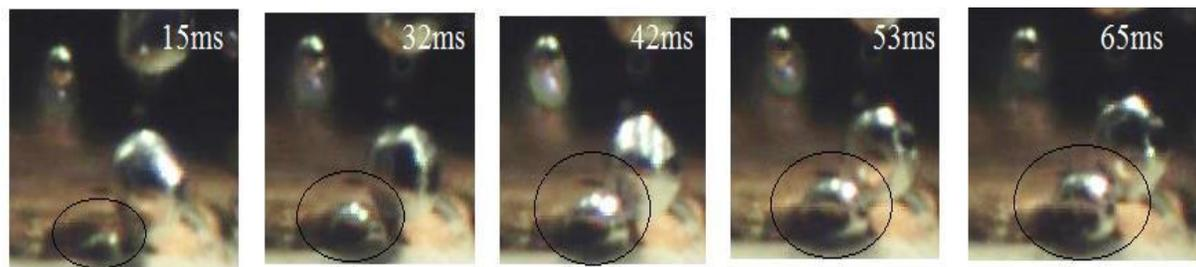
**Fig. 11** Bubble life cycle at f=2Hz, a=2.5mm at wall super heat 14.8°C
