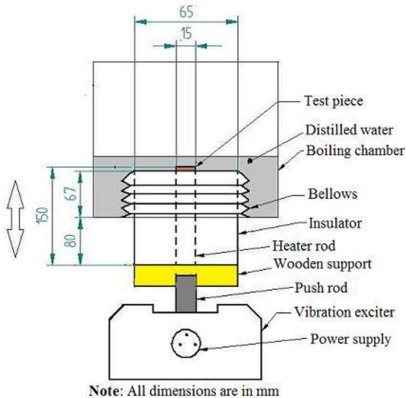
Fig. 3 Vibration arrangement
