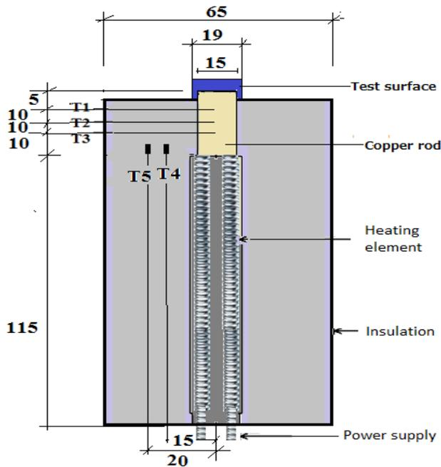
**Fig. 2 Details of heater assembly**
