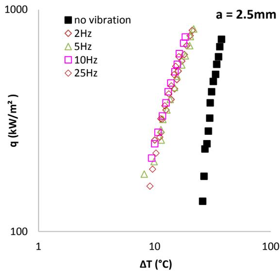
Fig. 8 Effect of frequency of vibration on boiling curves
