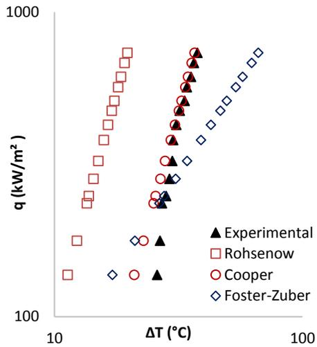
**Fig. 5** Experimental and predicted boiling curves of plain surface
