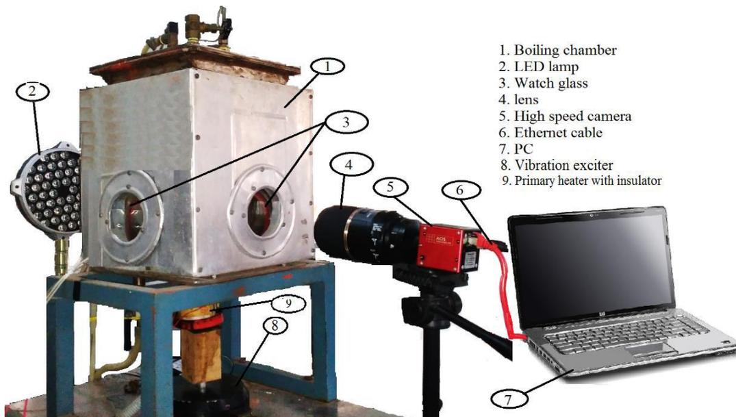
Fig. 4 Visualization of boiling process
