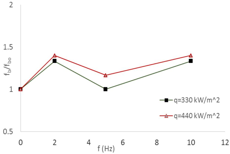
**Fig. 17 Normalised bubble frequency v/s frequency of induced vibration**
