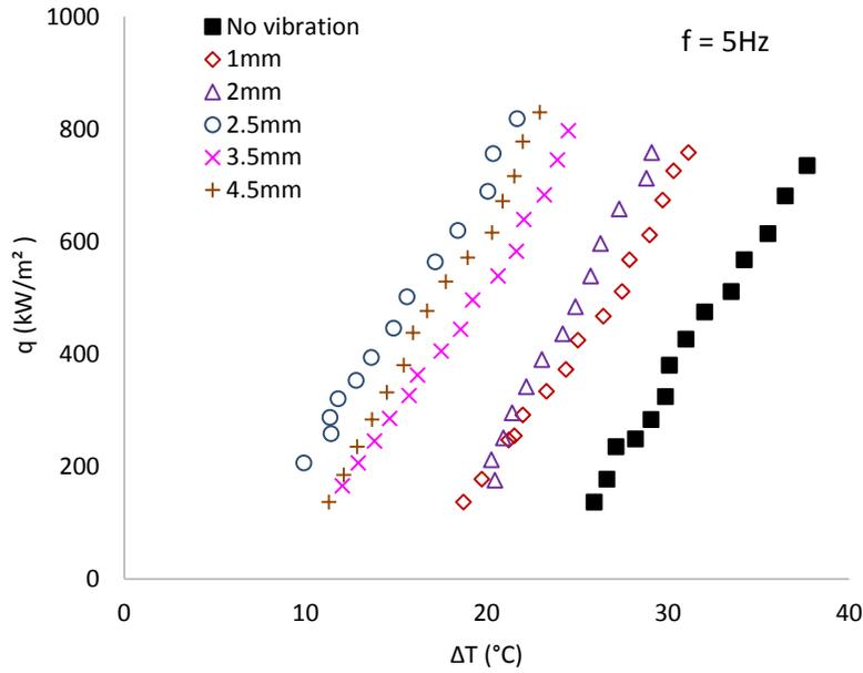
**Fig. 9** Effect of amplitude of vibration on boiling curves
