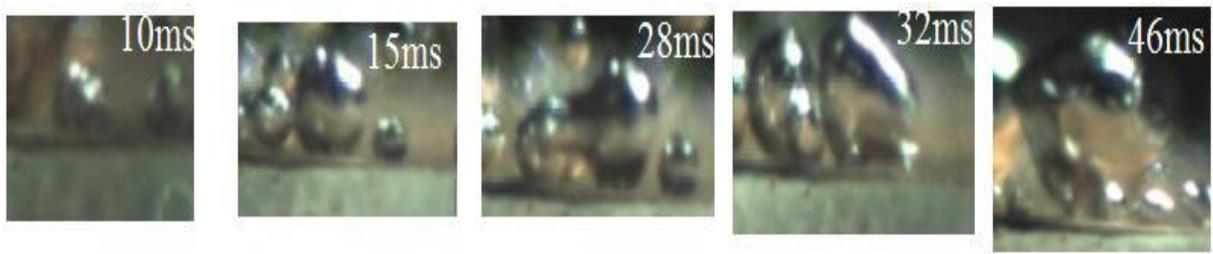
Fig. 12 Bubble life cycle at  $f=5\text{Hz}$ ,  $a=2.5\text{mm}$  at wall super heat  $13.2^\circ\text{C}$
