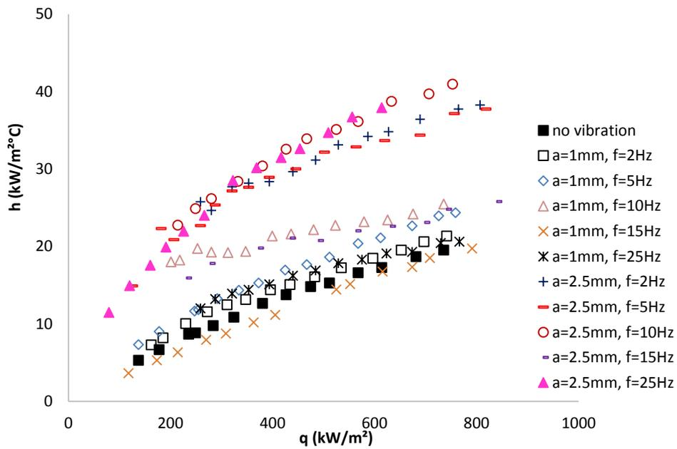
Fig. 7 Heat transfer coefficient v/s heat flux
