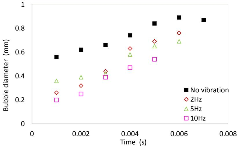
Fig. 14 Instantaneous bubble growth rates at constant amplitude 2.5mm
