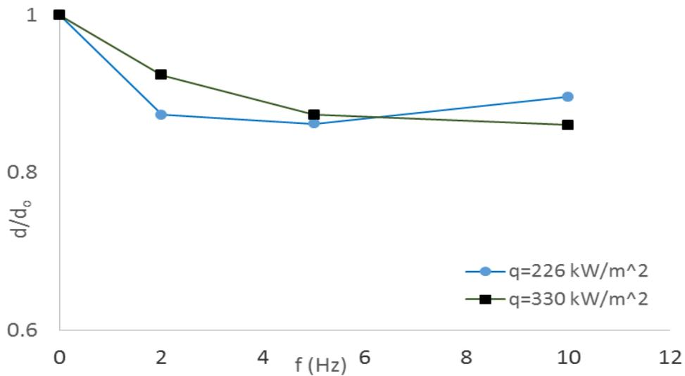
**Fig. 16** Normalised bubble departure diameter v/s frequency of induced vibration
