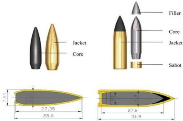
Figure 1: Original dimensions of 7.62\*32 bullets with body parts [4]
