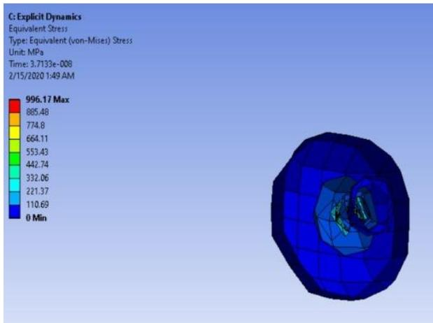
**Fig 11: Equivalent Stress of Bullet 2 Isosurface view**
