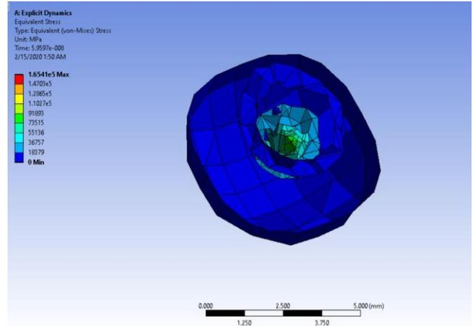
**Fig 12: Equivalent Stress of Bullet 4 Isosurface view**
