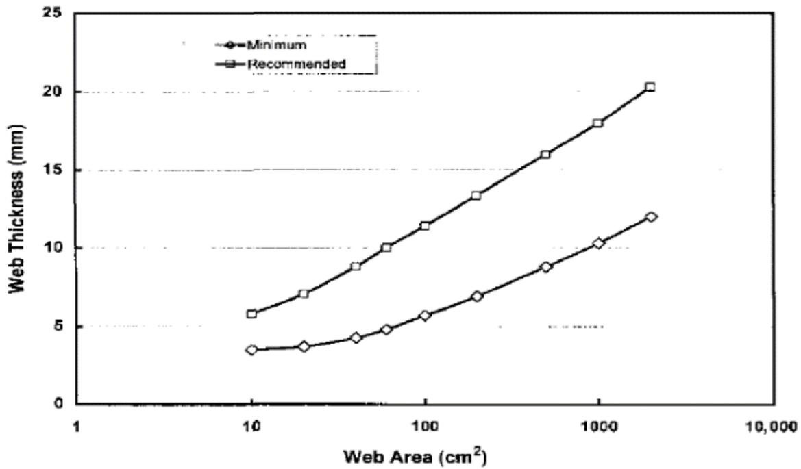
Fig 3.1 Web thickness related to projected area
