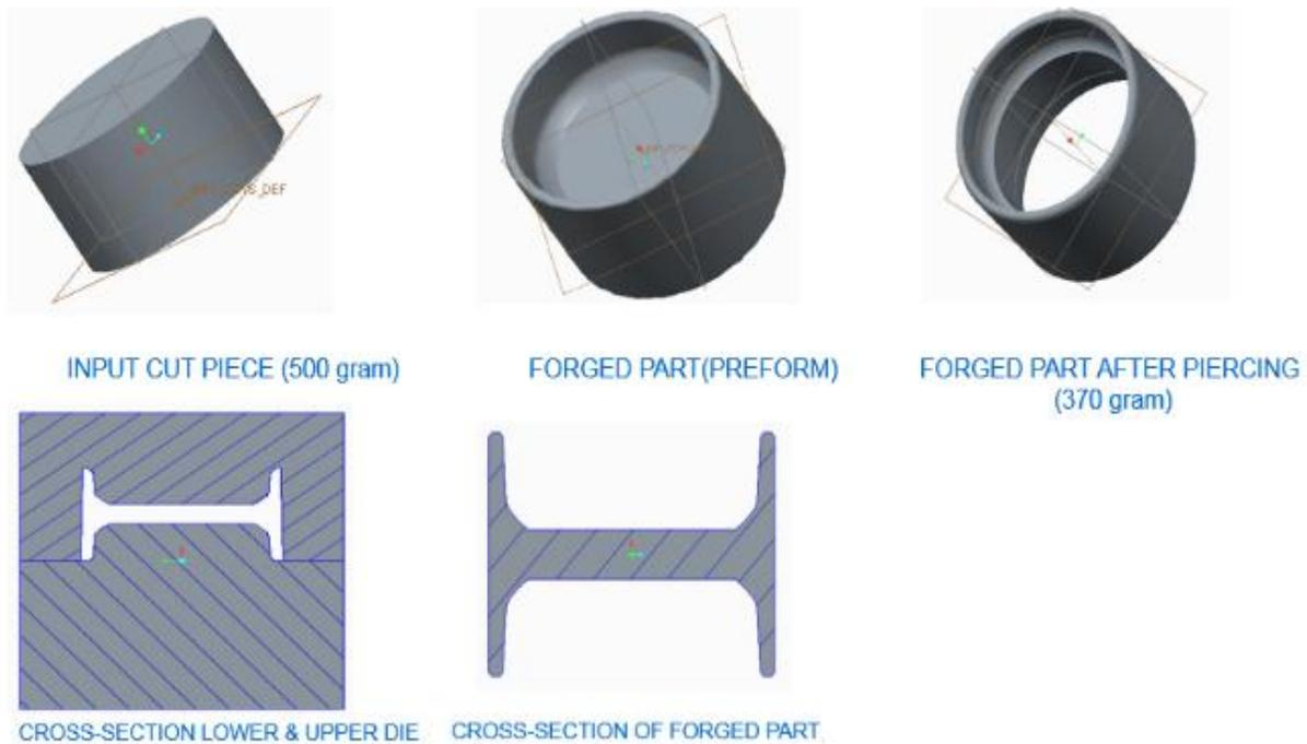
Fig 3.2 Stepwise present forged part and dies
