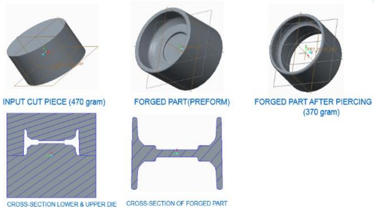
Fig 3.2 Stepwise proposed forged part and dies
