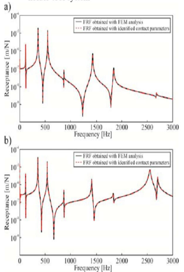
Fig. 3. FRF of the spindle-holder (a) and spindle-holder-tool (b) system with identified contact parameters
