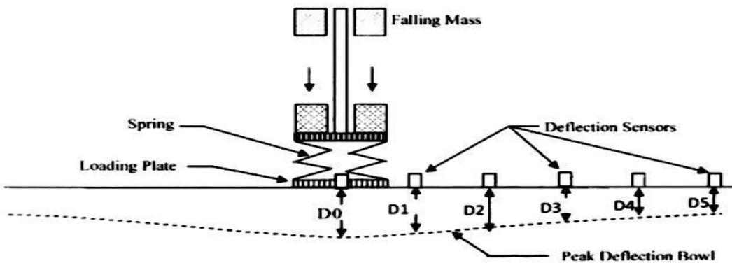
Figure 1 Working Principle of Falling Weight Deflectometer with deflection bowl
