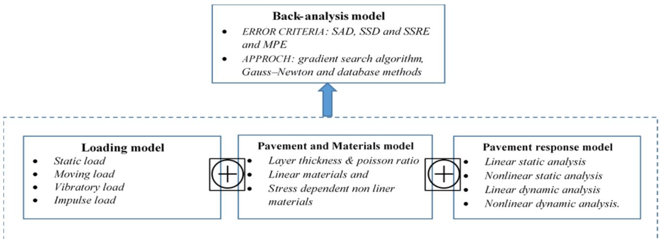
**Figure 3 components of back calculation**
