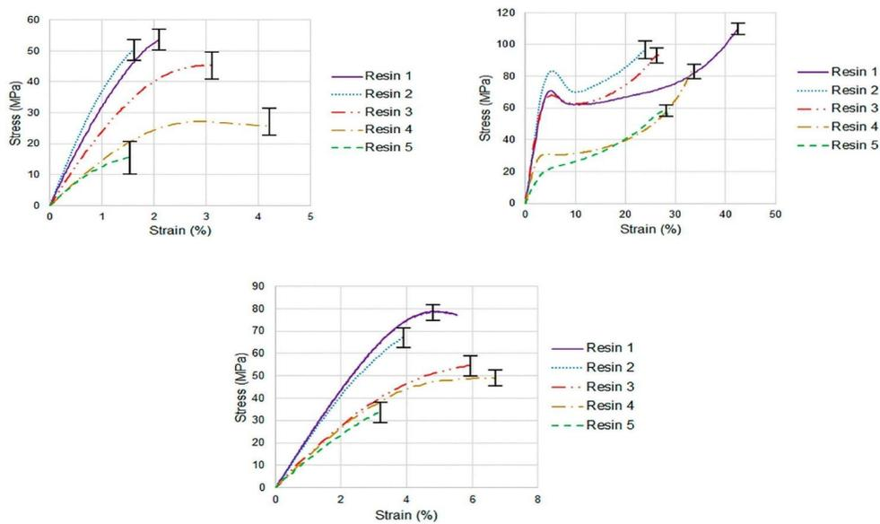
**FIGURE 2. TENSILE, COMPRESSION AND FLEXURAL TEST RESULTS**
