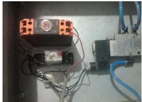
Fig: 7 Circuit board of controller with solenoid and Delay timer
