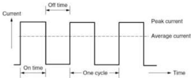
**Figure 2:** Typical EDM pulse current train for controlled pulse generator [2]
