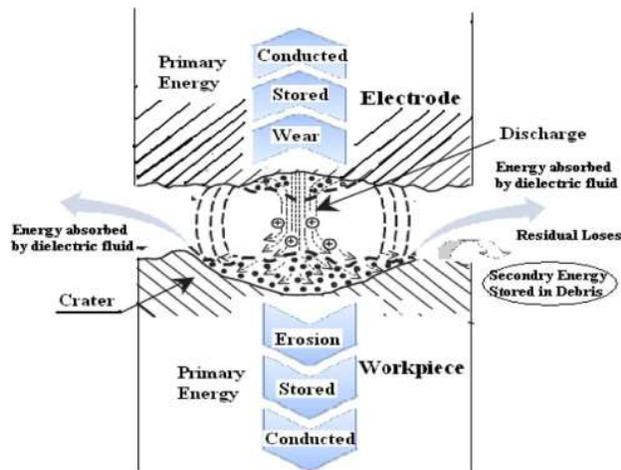
**Figure 3:** Distribution of spark energy evolved during EDM [3].
