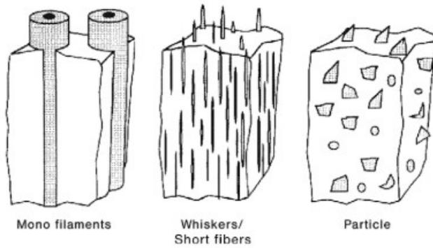
**Figure 1:** Types of MMCs on the basis of reinforcement [1]
