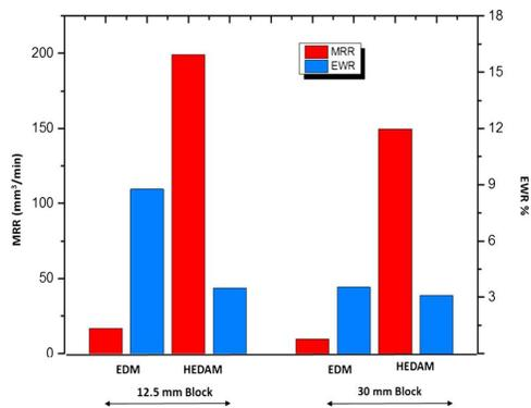
**Fig.4:** In this fig. shows the effect of EDM and HEDAM process for dissimilar thicknesses of the Inconel 718 work-piece [12]
