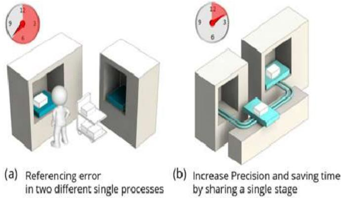
**Fig. 2** In this activity shows the Referencing issues in hybrid manufacturing. [8]
