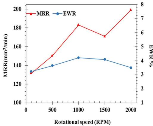
**Fig.3:** Effect of RPM on MRR and EWR at 50A and 8 MPa [11] Surface Roughness
