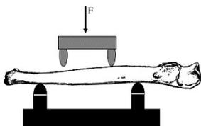
**Figure 3:** 4-point bending of a whole bone [8]
