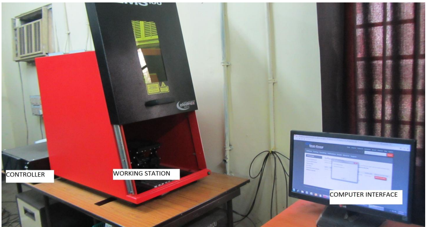
Fig. 2. Experimental Set-up for Laser Micro-drilling
