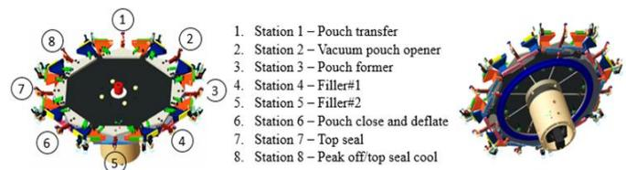
Fig. 1. Rotary Turret Assembly, Isometric View
