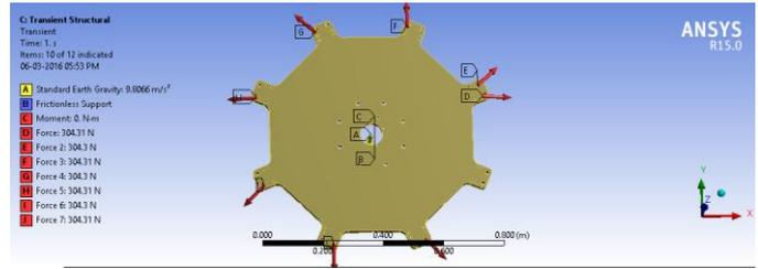
Fig. 6. Analysis setup for centrifugal force approach, Transient structural
