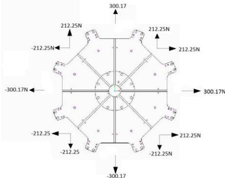
Fig. 2. X ,Y components of centrifugal force at eight different stations
