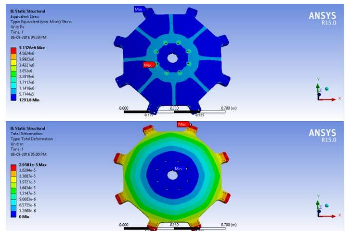
Fig. 4. Analysis results for static structural – von mises stress , total deformation
