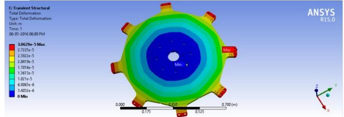
Fig. 7. Analysis results for transient structural – von mises stress , total deformation
