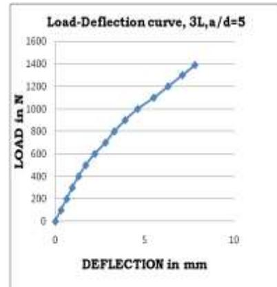
Fig.4 Load-Deflection curve of plate element ( $a/d=5$ )
