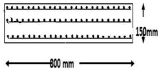
Fig.1 Details & Dimensions of the plate element
