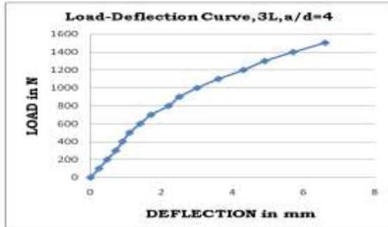
Fig.5 Load-Deflection curve of plate element (a/d=4)
