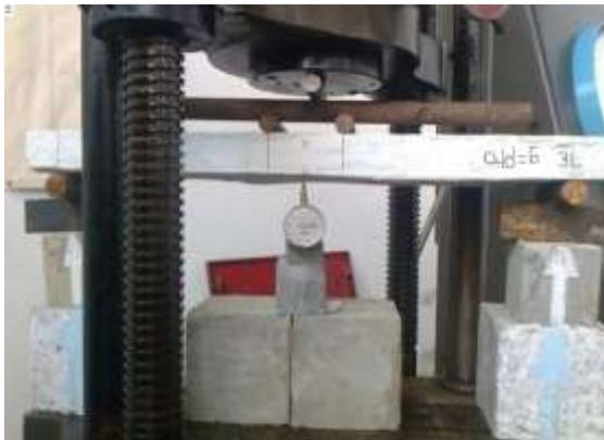
Fig.8 Plate Element Under Flexure Testing
