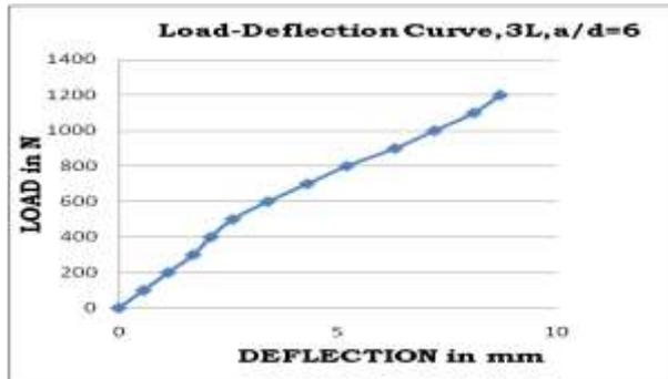
Fig.3 Load-Deflection curve of plate element ( $a/d=6$ )
