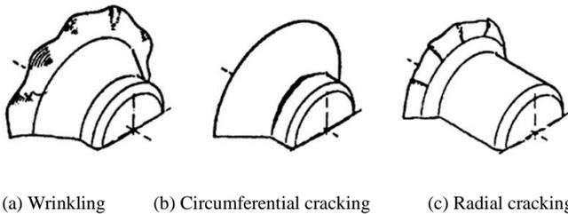
Fig. 1.3 Spinning failures
