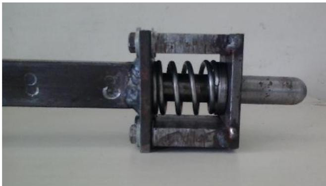
Fig. 3.1 Spring loaded tool
