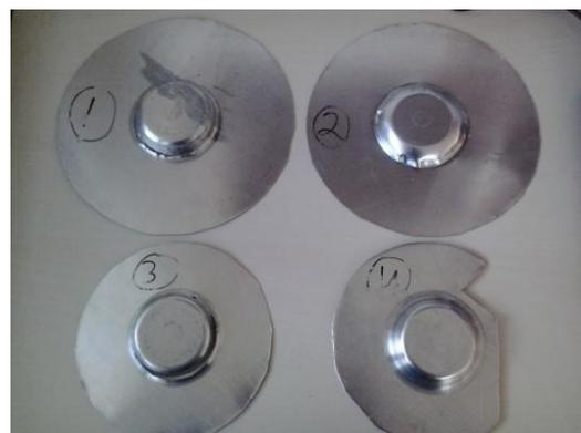
Fig 3.2 Pictorial view of spun parts
