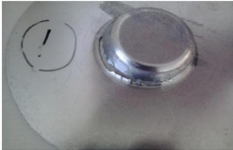
Figure 3.3 Circumferential cracking
