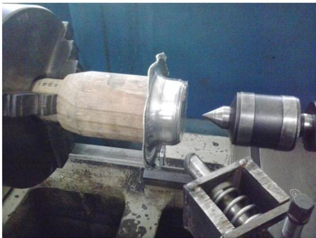
Fig 3.4 Wrinkling Failure
