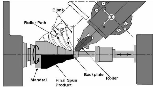
Fig. 1.1 Setup of metal spinning process
