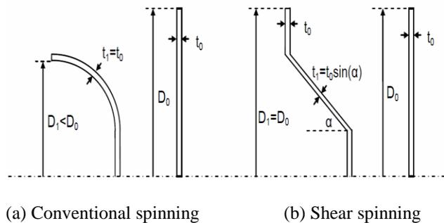
Fig. 1.2 Conventional spinning and shear spinning
