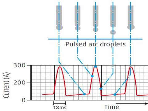
**FIG.2, Droplet Transfer System [24]**
