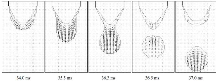
**FIG.8, Predicted droplet profile, melting interface, and velocity field in spray transfer mode**
