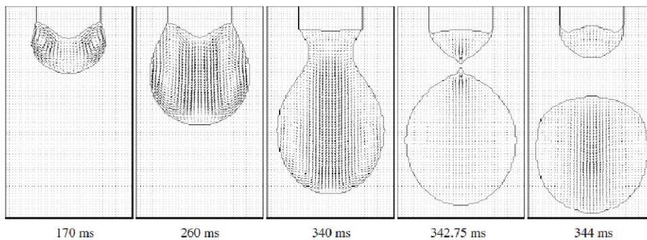
**FIG.7, Predicted droplet profile, melting interface, and velocity field in globular transfer mode**
