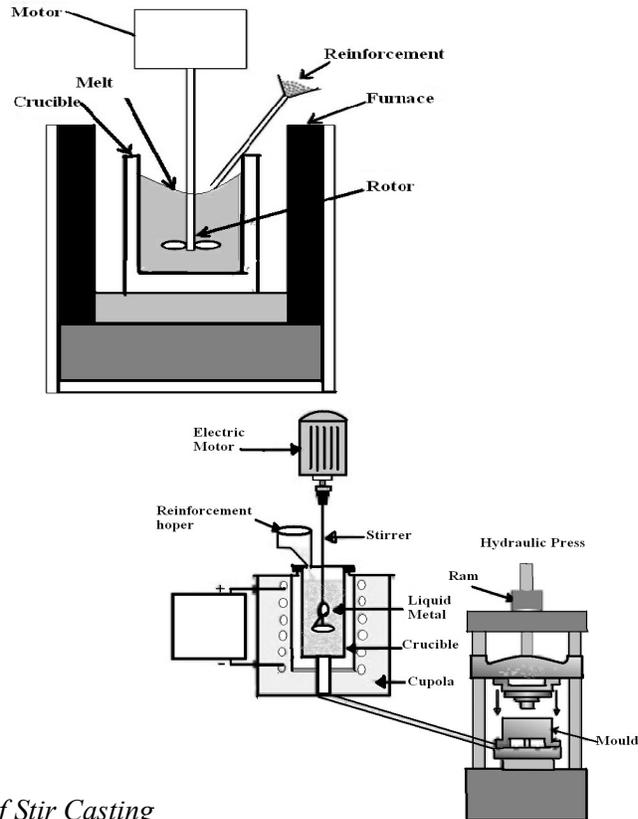
*Figure 2: Set Up of Stir Casting*
