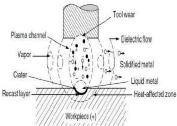
*Figure 1: Spark description of EDM process [1]*
