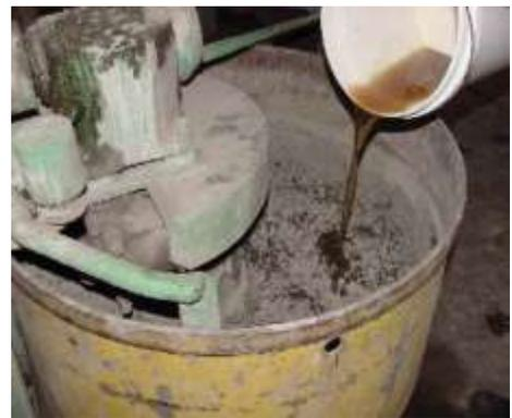
Fig.2 Adding liquid component in Pan Mixer
