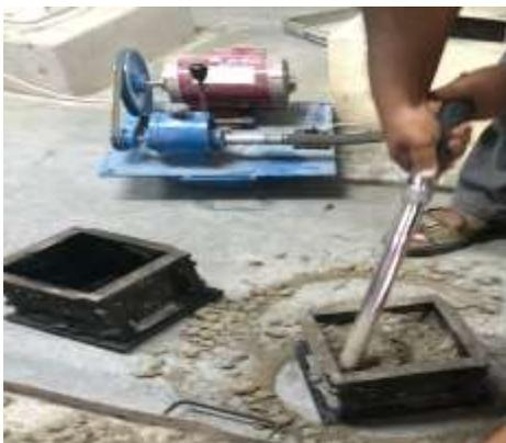
Fig.3 Compacting using vibrator
