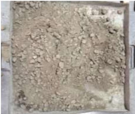
Fig.1 Mixture of CA, FA, and Fly ash
