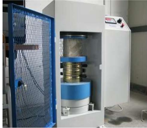
Fig.6 Compression Testing Machine
