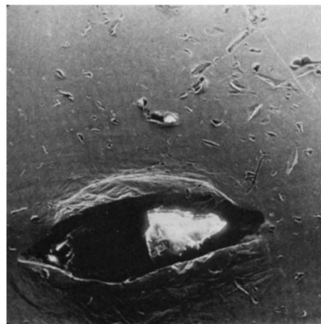
Fig.1. Primary indentation surrounded by secondary damage of H46 steel.
